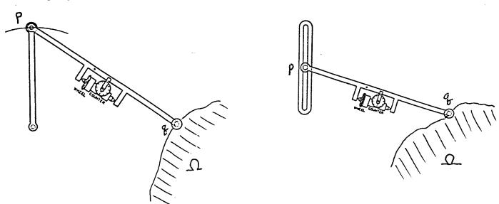
When the planimeter is used to measure the area of  $\Omega$ , it mechanically integrates (1). Since it returns to its original position,  $d\theta$  integrates to  $2\pi n$ , where n is the number of rotations made by the planimeter. Thus we have
