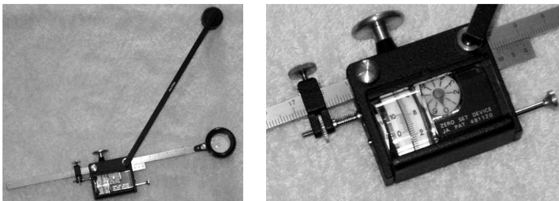
Figure 9. Commercial planimeter and the scale on its measuring wheel.
