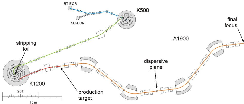
Figure 1.2: The coupled cyclotrons and the A1900 fragment separator.
