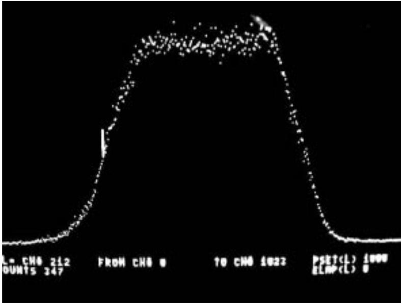
Figure 6.2: A pulse height spectrum of the time difference generated by the cosmic-ray muons. In this run the discriminator levels were set almost at zero. For higher discriminator threshold settings the edges of the “rectangle” should be sharper.
