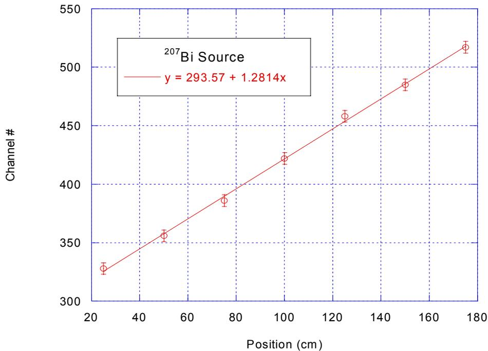
Figure 6.4: A plot of channel number vs. position of a  $^{207}\text{Bi}$  source along the bar.
