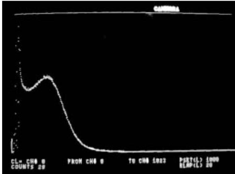
Figure 4.4: The pulse height spectrum from one phototube for a  $^{137}\text{Cs}$  source placed at the center of the bar. Amplifier gain was 900.
