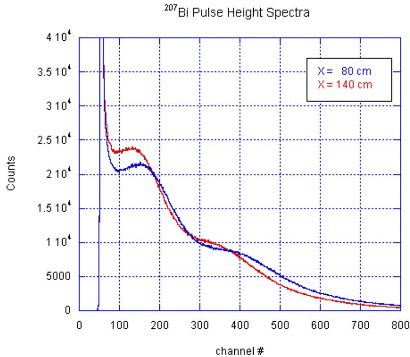
Figure 5.1 : A <sup>207</sup>Bi source is placed on top of the detector bar at a position  $x$  from the active phototube as shown in the schematic at the top. The plot below shows the raw pulse height spectra for  $x = 80$  cm (blue) and  $x = 140$  cm (red). Notice the peaks shift to a lower channel number as  $x$  increases.
