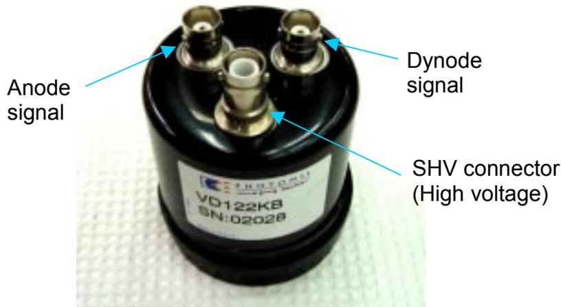
Figure 4.2: The connectors on the voltage divider.
