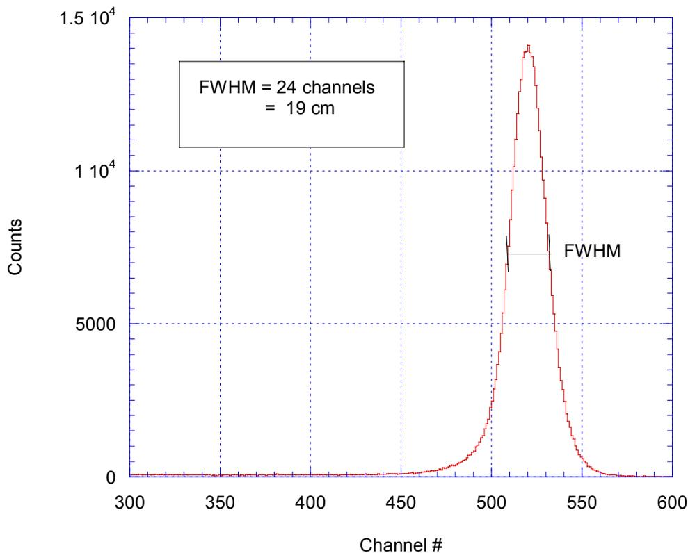
Figure 6.5: In the top diagram the source emits gamma-rays in many directions. The individual events are spread out in position along the bar giving rise to a large spread in the FWHM of the peak as shown in the plot.
