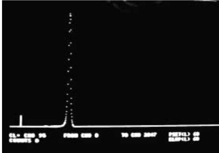
Figure 6.3: A pulse height spectrum of the timing difference with a  $^{207}\text{Bi}$  source placed at 25 cm from the left bar end.
