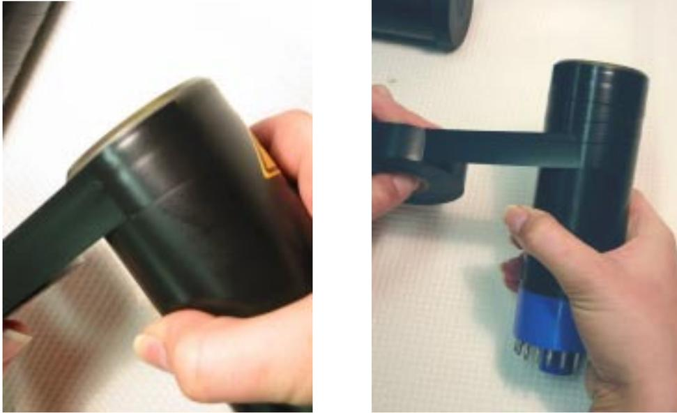
Figure 3.3: Black electric tape is wrapped around the phototube. Begin at the top of the tube (left) and wrap in a spiral pattern (right).
