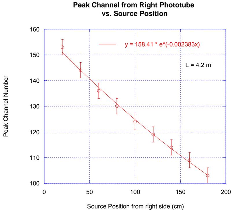
Figure 5.2: A plot of peak channel number vs. the source position using  $^{207}\text{Bi}$  source. An exponential fit yields a value of 4.2 meters for the attenuation length.
