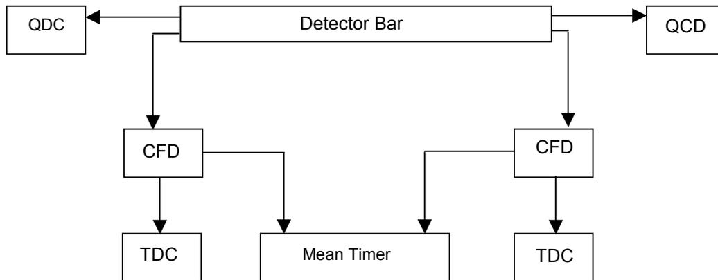
Figure 2.3: A simplified schematic of the MoNA detector module electronics.
