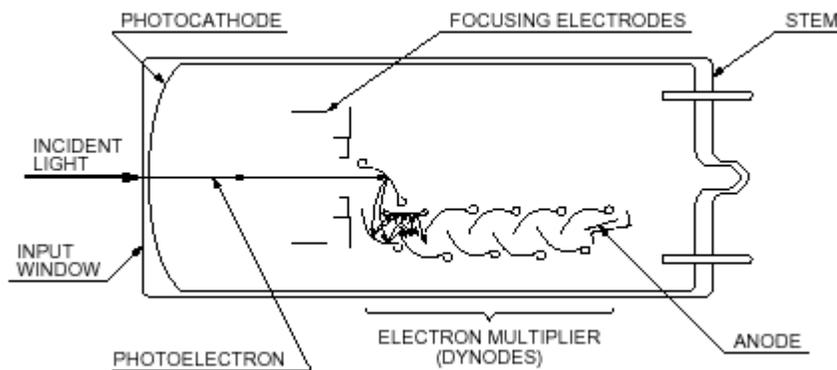
Figure 2.2: A schematic drawing of a typical phototube.
