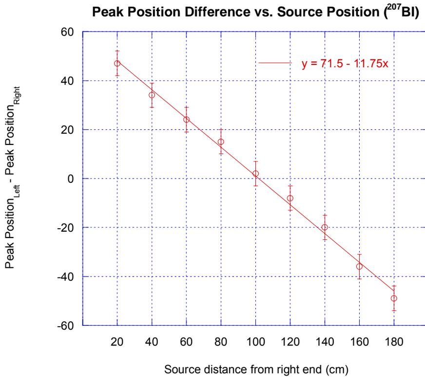
Figure 5.3: A plot of peak channel difference vs. source position using  $^{207}\text{Bi}$ . A linear fit yields  $y = -11.75 X + 71.5$ .
