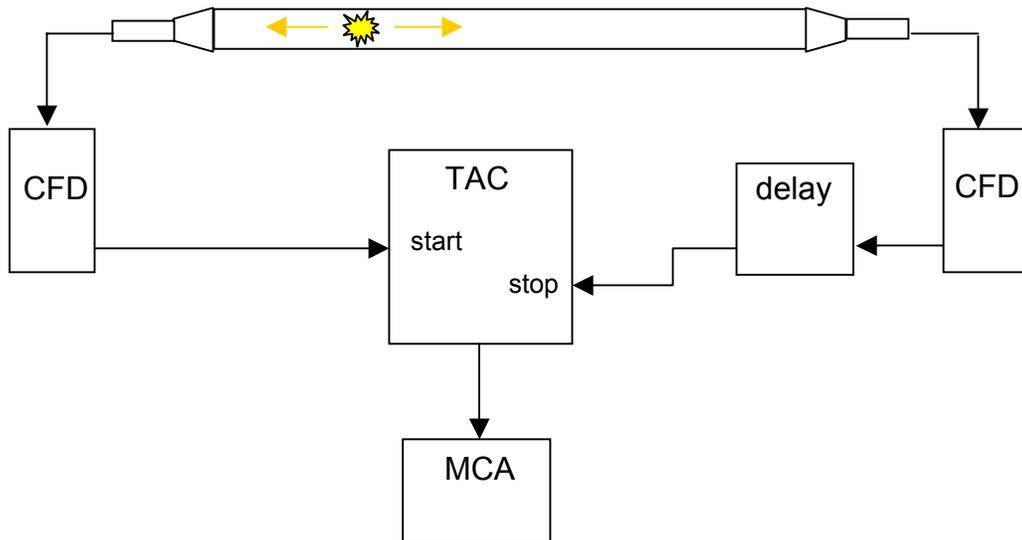
Figure 6.1: A schematic for a basic electronic setup to measure the difference in signal arrival time at the bar ends.
