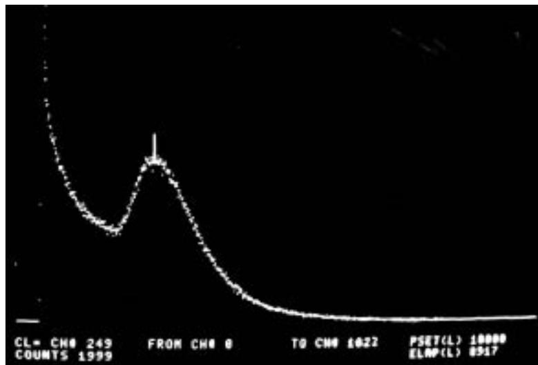
Figure 4.1: The cosmic ray spectrum taken from a detector bar. Notice the prominent peak corresponds to an energy deposition of 20.7 MeV in the bar.
